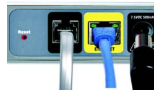
Figure 3-5: Connect to the Power Port
